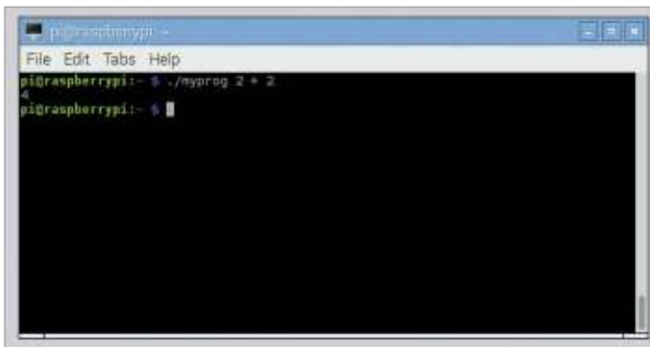
**Left** The calculator reads the two values and the operator from the argv array and prints the result
