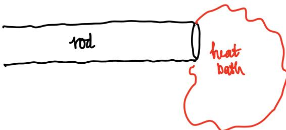
From the previous problem the heat flux leaving the rod is equal to the flux entering the heat bath.
